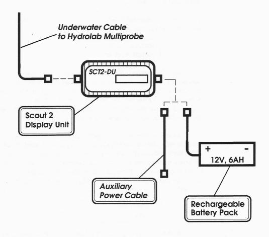
Figure 1.1 Scout 2 System Components
