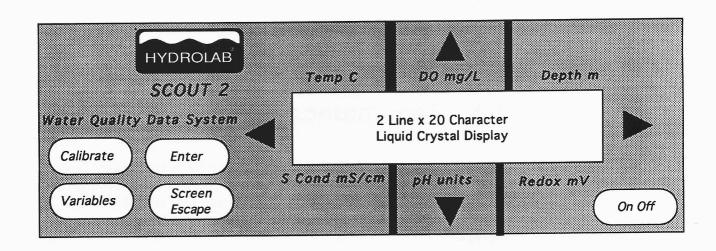
Figure 1.2 Scout 2 Display Unit Panel Keys
